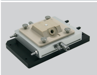
Linkam Temperature Control Stage (RT to +600°C)
